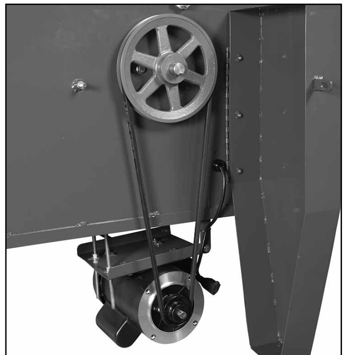
Blade shaft to motor pulleys and belts
