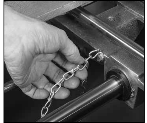
Slab saw automatic shut-off chain & adjustment to carriage hook
