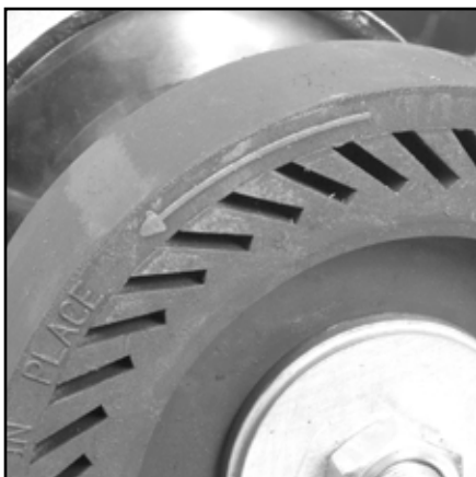
Fig 59 - Arrow on drum indicates direction of rotation
