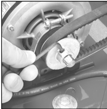
Fig 65 - Motor arbor shaft pulley.
