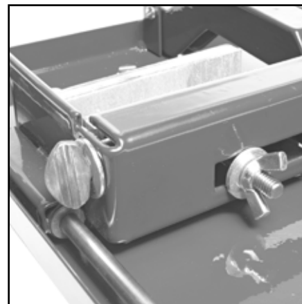
Fig 13 - Cross feed lock (right) and cross feed thumb screw (left)
