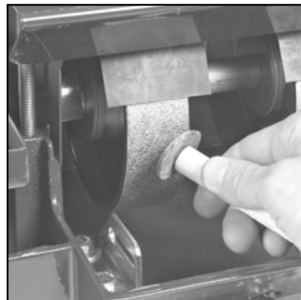
Fig 34 - Grinding with tool rest removed
