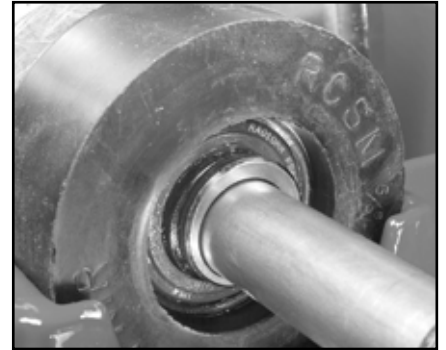
Fig 30 - Bearing correctly installed
