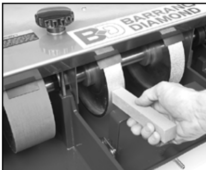
Fig 14 - Carbide stick applied to diamond wheel
