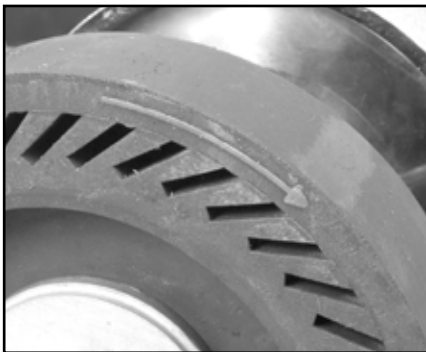
Fig 37 - Arrow on drum indicates direction of rotation
