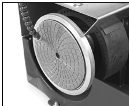
Fig 21 - Polishing pad centered on flat aluminum disc
