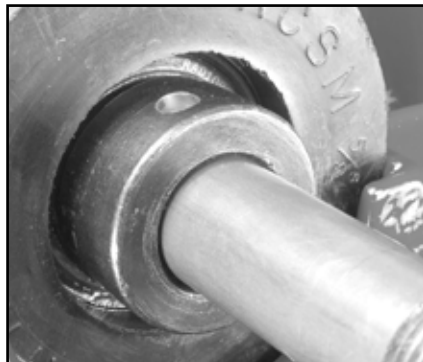
Fig 32 - Bearing collar correctly installed
