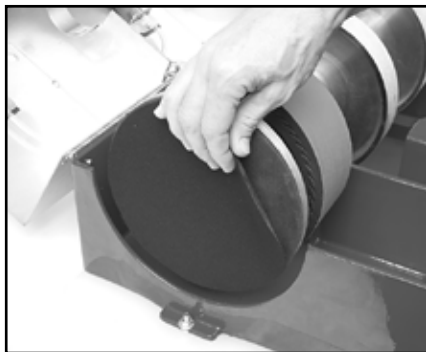
Fig 16 - Polytex pad being applied to the convex polishing disc
