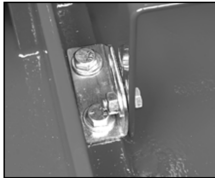
Fig 12 - Tool rest positioning bolt
