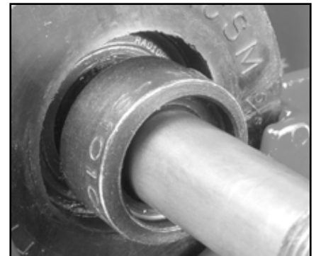
Fig 33 - Bearing collar incorrectly installed
