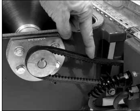
Fig. 7. V-belt correctly tensioned
