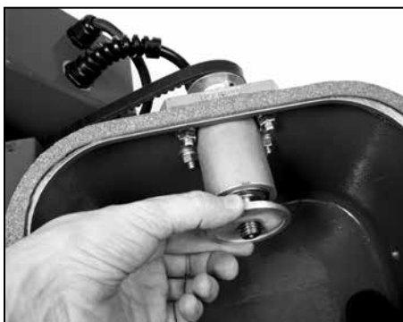
Fig. 36. Convex or recessed side of blade flange
