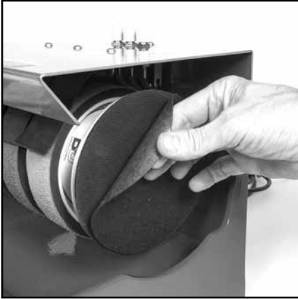
Fig 13 - Polytex pad being applied to the convex polishing disc
