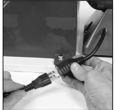
Fig 10 - Electrical outlet for water pump
