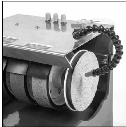
Fig 17 - Position water nozzle on pad
