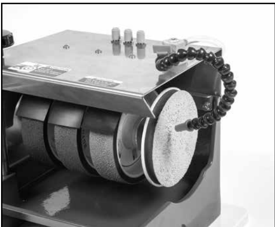
Fig 19 Loc-Line nozzle placement -
