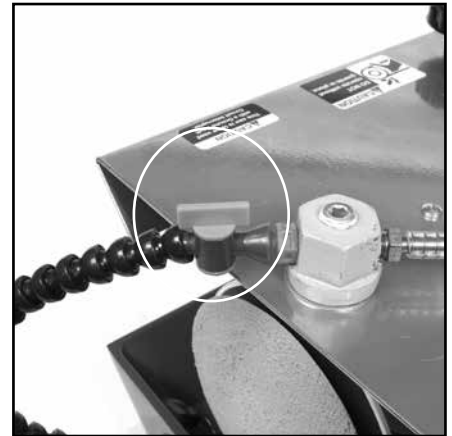
Fig 18 - Water flow adjustment valve
