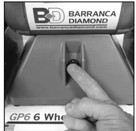
Fig 4 - Power switch in the ON position
