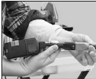
(B) Plug-in the power cord using a GFCI.
