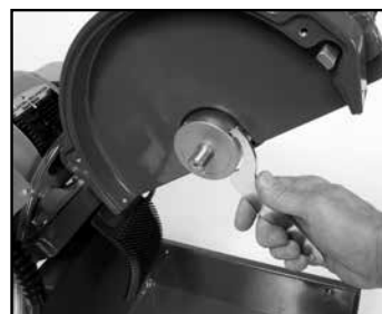
(F) Locate the inner flange wrench retaining holes.
