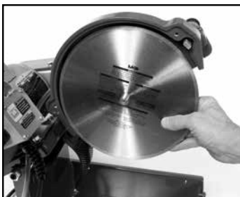
(G) Install diamond blade. Verify the blade is seated on the blade shaft.
