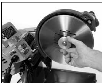
(H) Install outer flange. Ensure the diamond blade rotational arrow matches the direction of the blade guard arrow.
