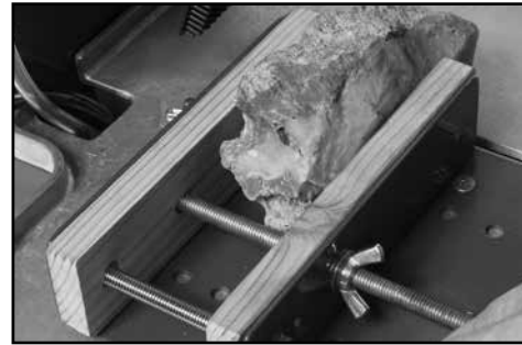
(B) With material in vise, tighten wing nuts until front and back jaws are tightly securing material.
