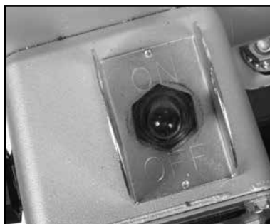
(E) Turn saw OFF immediately after finishing cutting.
