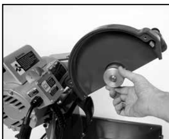
(E) Remove the outer flange.
