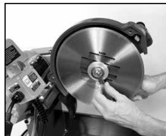
(I) Tighten retaining nut.
