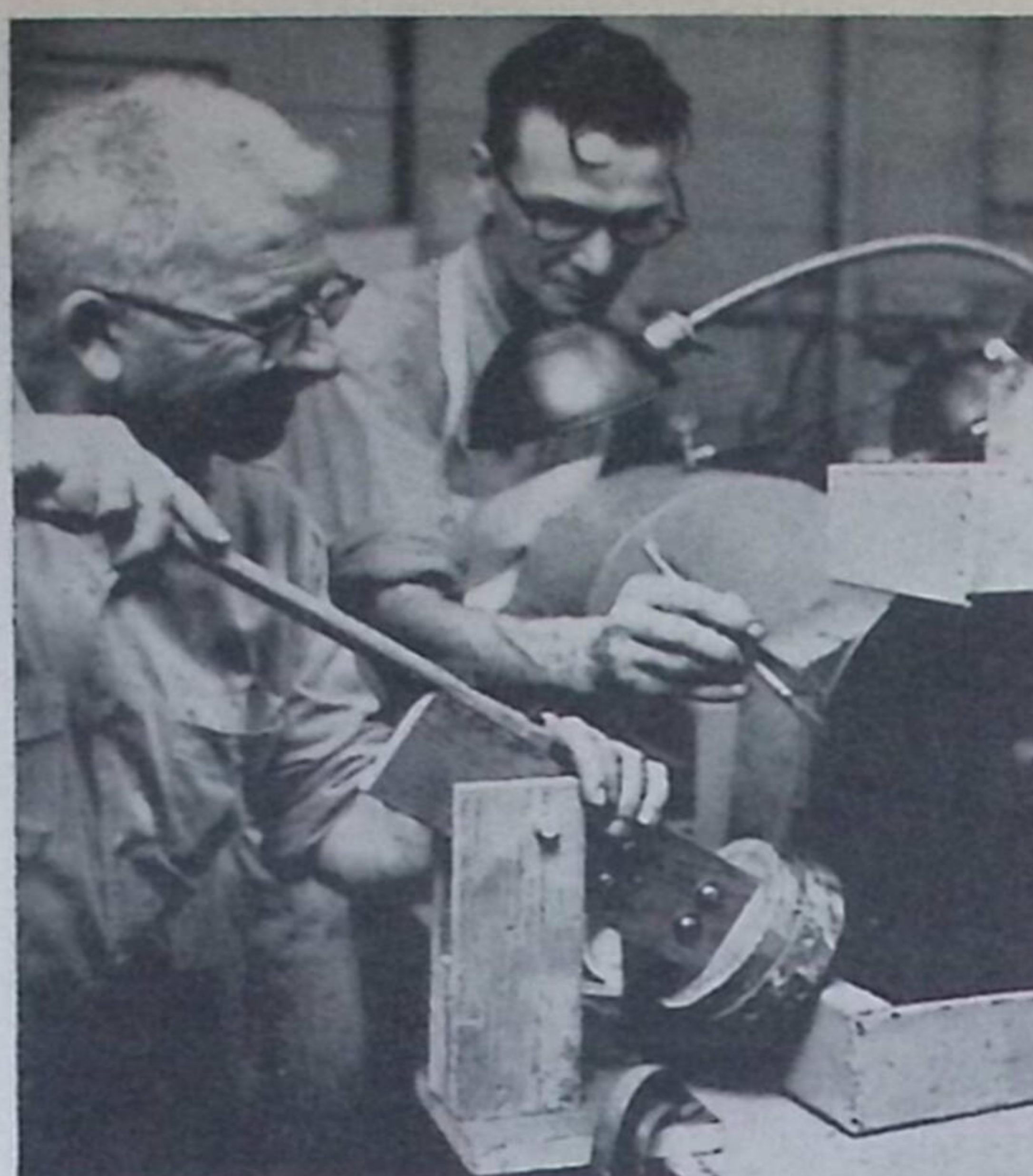
On left above: Alden Clark using a special device for sawing the curved face on pendulum bob. Robert Hardenbrook puts coolant on the saw.
