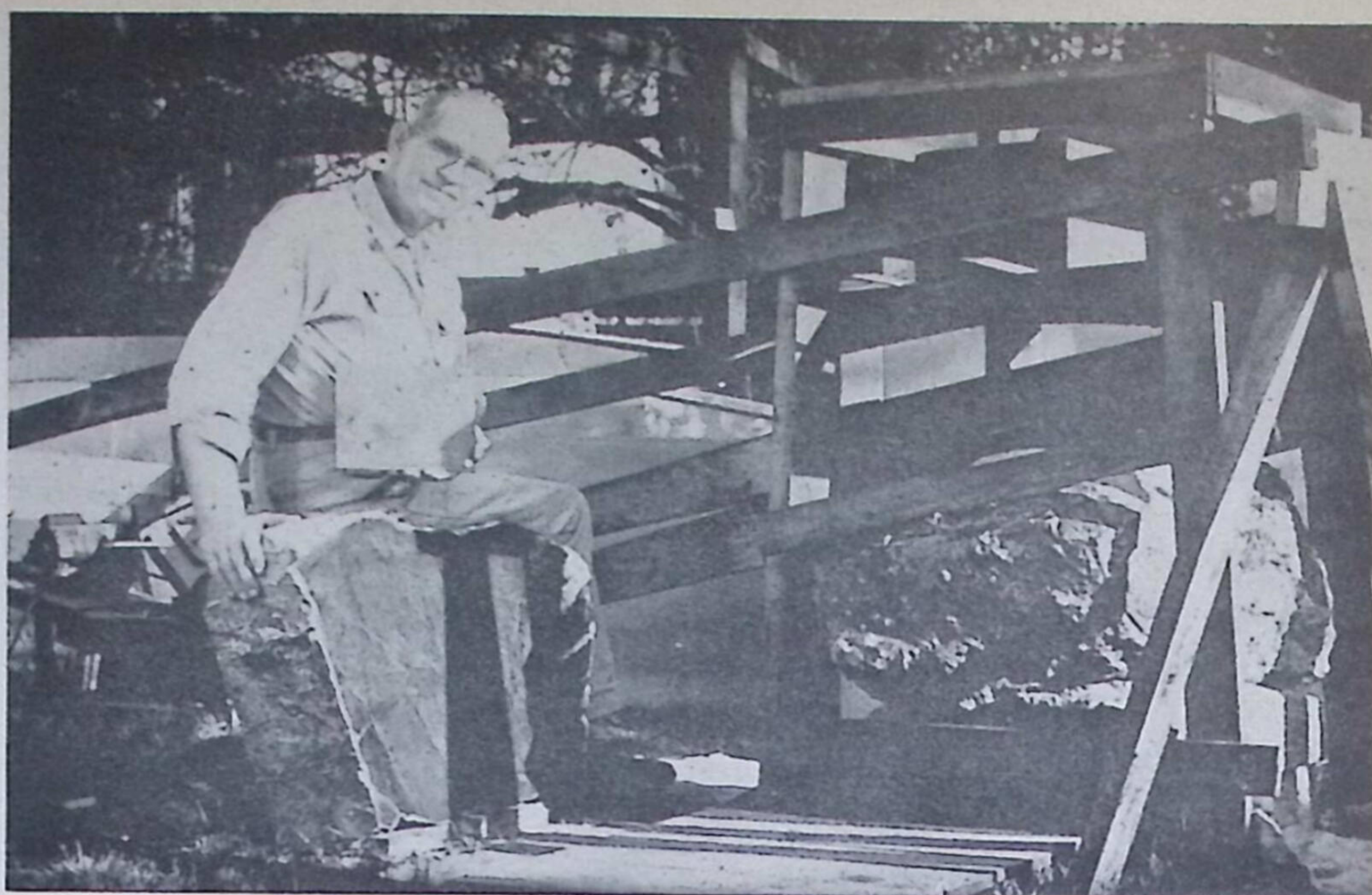
L. J. Bergsten cutting a one-ton jade boulder on a mud saw in his backyard.
